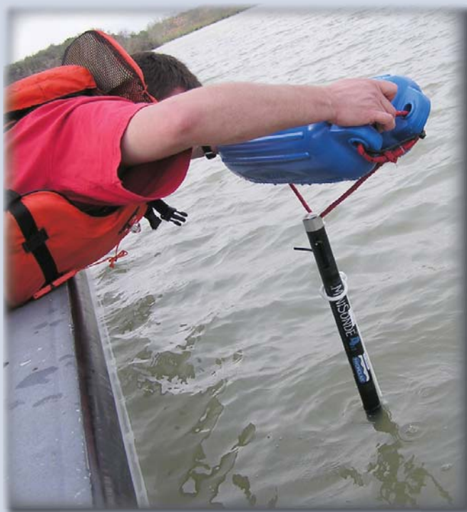
Deploying 24-hour DO monitors
